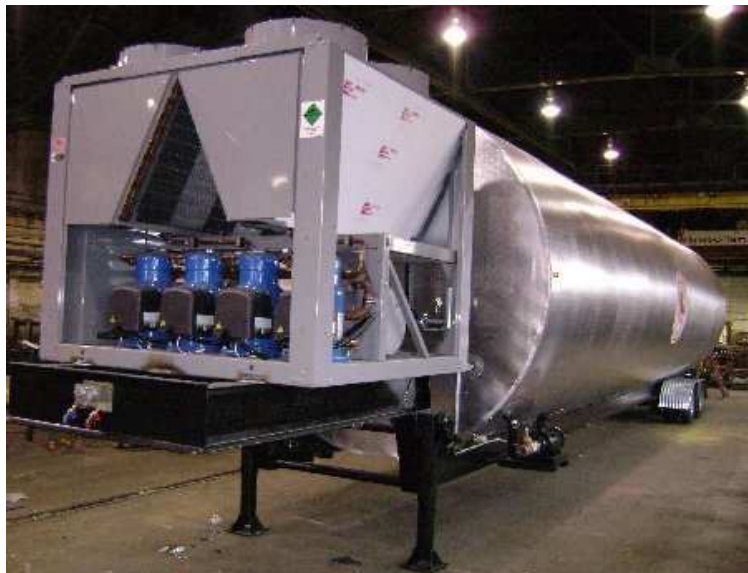
30,000 gal portable chiller unit with 80 ton chiller
