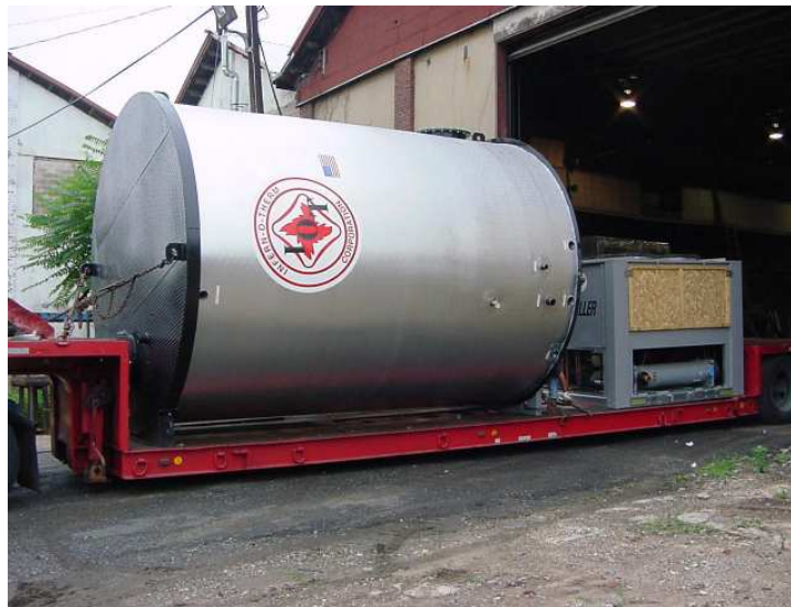
40 Ton Infern-O-Therm Chiller w/ 10,000 gal Vertical Storage Tank
